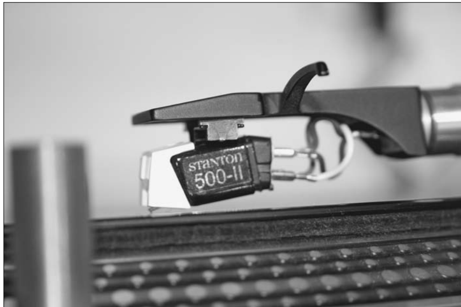
Figure 6-2: A Technics headshell with Stanton 500AL attached.
