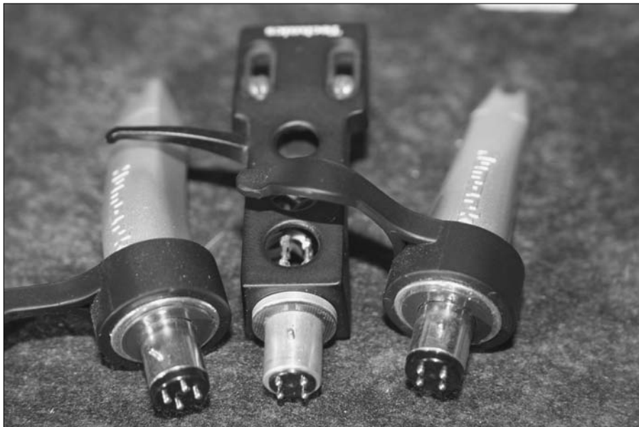
Figure 6-1: The same connection on the back of different cartridges.
